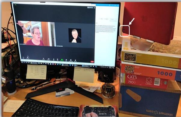
A test-taking desktop machine using an iPad as the camera and microphone. Notice the homebrew “boxes” stand for the tablet. The iPad is turned around so it uses its higher-quality rear camera.
