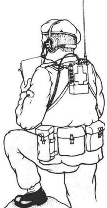
UK Military – narrow-band FM VHF man-pack radio that operates from 36-57MHz in 2KHz steps, total of 841 programmable channels with 2 Watts output.
