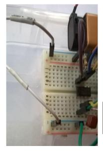
Connect the black wire from the battery clip to the UNUSED "-" blue power rail on the opposite side of the breadboard that you used for the circuit. Then connect the wires from the key to each blue "-" power rail on the breadboard. When the key is closed, the circuit is completed!
