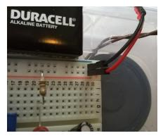
Black battery clip lead ("-") $\rightarrow$  <u>UNUSED</u> blue power rail ("-") Each key wire  $\rightarrow$  blue power rails ("-") on each side of breadboard
